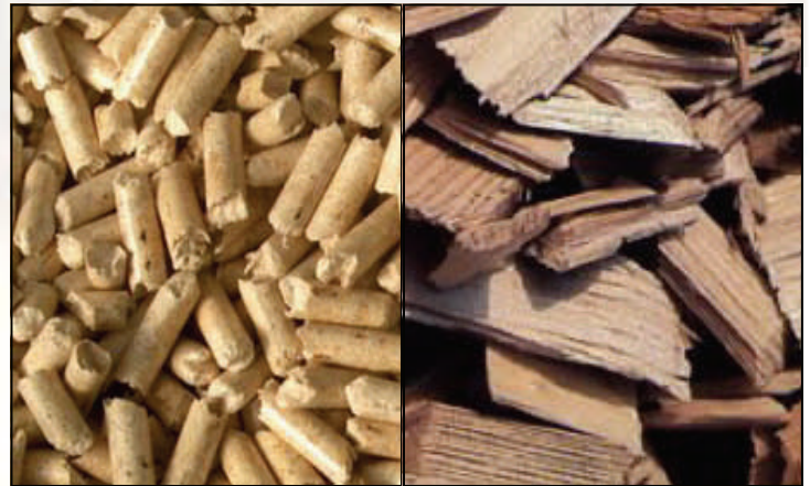
Typical wood pellets on left and wood chips on right.
